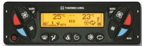
Driver's panel on the dashboard (188 x 59 mm)
